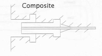
Figure 2: Ferrule after embedding and removal of the mold.
