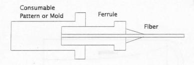
Figure 1: A ferrule with attached consumable pattern, or mold.
